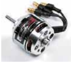
Motor Brushless Outrunner Motor Voltage: 6.4~12.6V (2~3S LiPoly) RPM / V: 1130kv Max current: 17A
