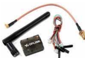
Oplink Mini Ground Station 433MHZ RF link 100mW RF Output Micro-B USB
